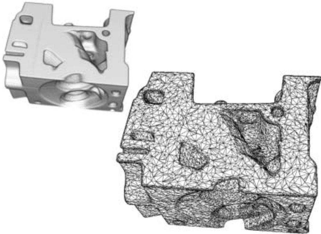
*Fig. 203 Volumetric data set of a cylinder-head and an extracted polygonal model (STL file).*
